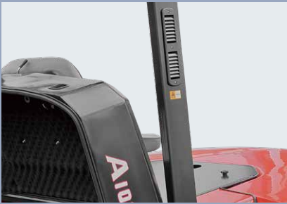
The engine's air intake pipe is provided as an independent channel in a high position to effectively prevent dust from being sucked in
