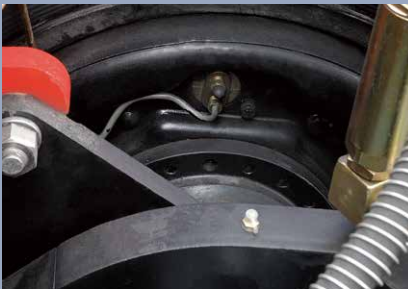
A drum brake is used, which is safer, more reliable, and easy to maintain
